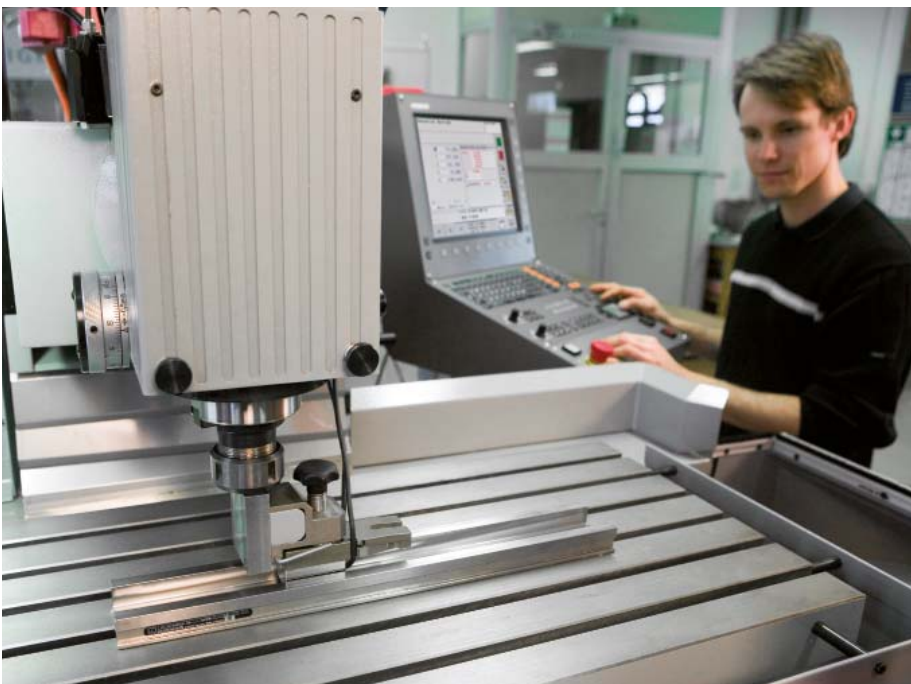
Determining the positioning accuracy with a VM 182
