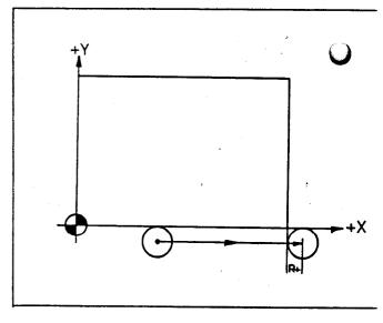
If R- is programmed, then the traversing distance is <u>reduced</u> by the size of the tool radius. e.g. interior contour.
