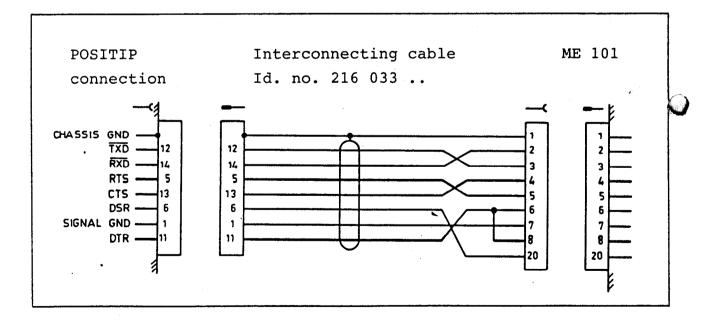
The following connector layout is suitable for the connection of a typical peripheral device (e.g. printer with tape reader/punch) to the ME 101.
