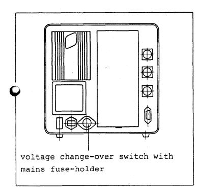
The POSITIP VRZ 965 is set in the works to 220V; this may be changed to an operating voltage of 100, 120, 140, 200 or 240V.
