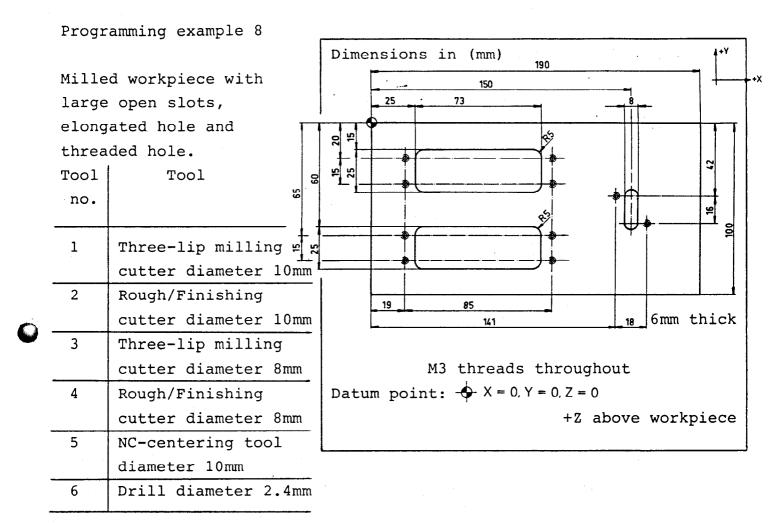
Material: Cast aluminium Thickness of workpiece: 6mm
