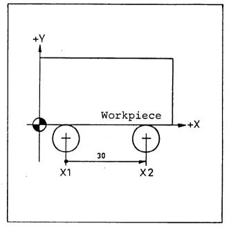
The tool is in position X1=10mm The machine axis is to be traversed to position X2=40mm Both dimensions are relative to the (absolute) workpiece datum point (marked by --). The tool is in position X1. The machine axis is to be traversed by 30mm to position X2. With incremental dimensions, the path to be traversed is not relative to the workpiece datum point, but is instead relative to the position that was reached after the last positioning.
