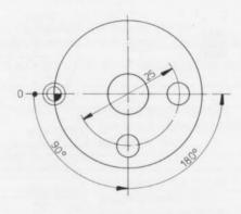
Incremental dimensions refer to the previous position of the rotary table or tool.
