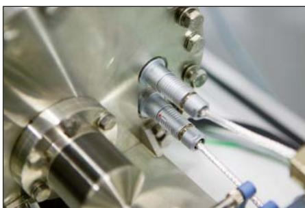
Vacuum-compatible housing lead-throughs
