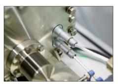
Vacuum-compatible housing lead-throughs
