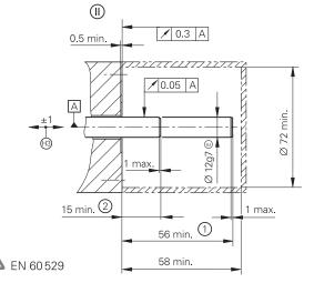
mm  $\Box$ Tolerancing ISO 8015 ISO 2768 - m H < 6 mm: ±0.2 mm
